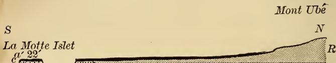
FIG. 7.—Sections from La Motte Islet to Mont Ubé, Jersey. a' , rubble drift, composed of granitic and diorite débris from Mont Ubé, in a brick earth or loess, covered by a sandy earth and soil; c , raised beach—only portions of this remain. The elevation of Mont Ubé is 150 feet. La Motte Islet is 1,000 feet from the shore, and is of only a few acres in extent and accessible at low water. It consists of a base of diorite, capped by the remains of an old beach, overlaid by a mass of rubble drift or head , the section of which is very similar to that shown in Fig. 1, page 150. The distance to which this rubble drift is here spread out over a gentle slope from its source is too great to have been produced by snow slides.
